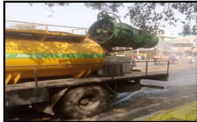
There is total 08 Water Sprinkler/Foggers (04-Truck mounted and 04 Tractor mounted) runs across the city, where each sprinkler sprinkled around 40 km of road per day. After passing the order by Hon'ble NGT dated 03.11.2023, the frequency of each Water Sprinkler has increased to around 55 Km per day. Now, the total length of the road being sprinkled around 440 km per day.
